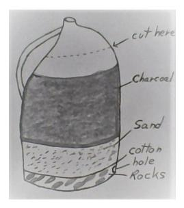
The top of the container should be cut off so that the cotton cloth can be spread on the bottom more easily. I'll leave enough space on top to let a whole glass of water in at a time. I'll probably use some sort of cork, in the bottom hole, so that some of the water can sit in the sand and rocks for a while before I drink it. I want it to gather as many minerals as possible.
